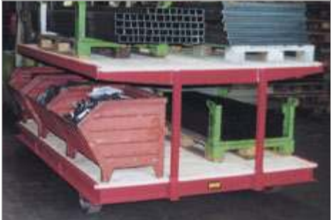
Additional loading surface in the form of a plug-in level
