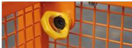
Anchorage point for protective equipment
