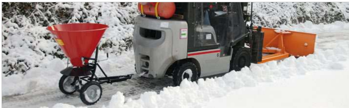
Type SCH-G in combination with type STW 100
