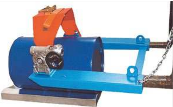
Setting down a drum on the shelf drum pallet type RP
