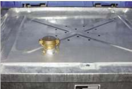
Filling tray and 2" tank truck coupling
