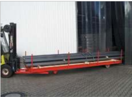
Transporting long materials; narrow turning circle due to pick-up
