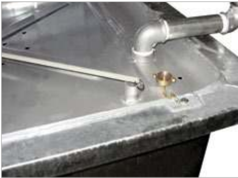
Dipstick to control the fill level
