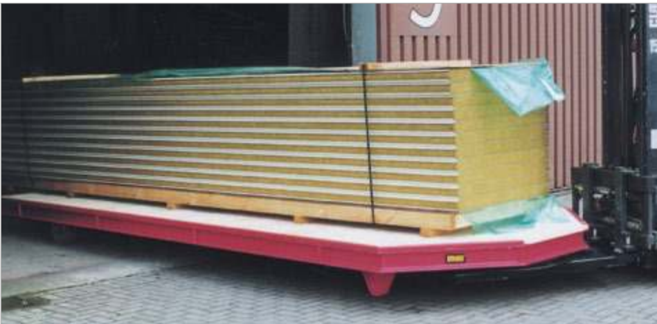
Transporting long materials; narrow turning circle due to pick-up
