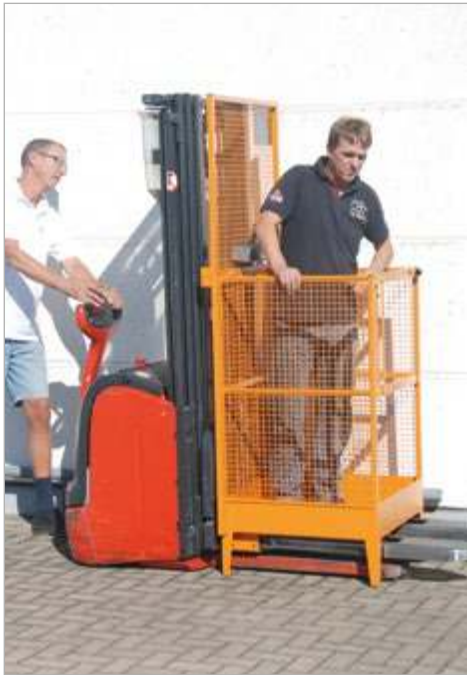
Type MB-I with straddle stacker
