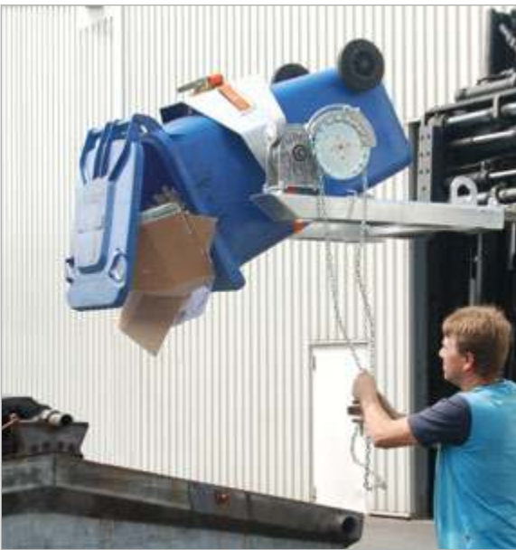
Type FLEX-K, emptying a 240 litre waste bin
